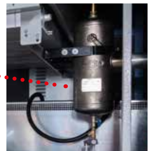
Condensate separator with automatic drain on models from 110 to 250 kW.
